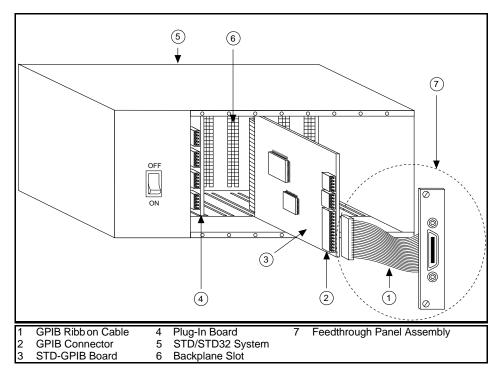
Figure 2-1. Installing the STD-GPIB Board
